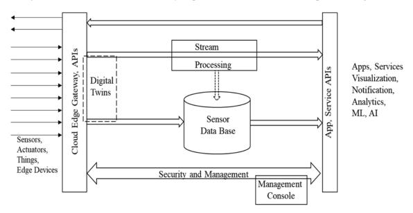
Figure 5 IoT Cloud Components
